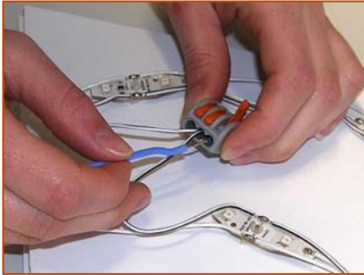
Electrical connection of the modules
